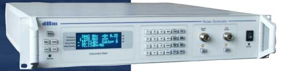
The WGN series instruments generate Additive White Gaussian Noise at levels that can be very accurately set in terms of noise power in a specified bandwidth. A 'smart" temperature stabilized attenuator with resolution better then 0.016dB provides extremely accurate and repeatable programming of output noise power.
